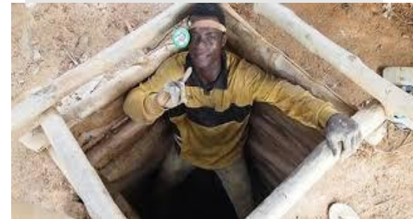
Underground Vertical Shaft for Auriferous Lodes and Quartz in Flat Plains beneath 15 m (Selati, 2016)
