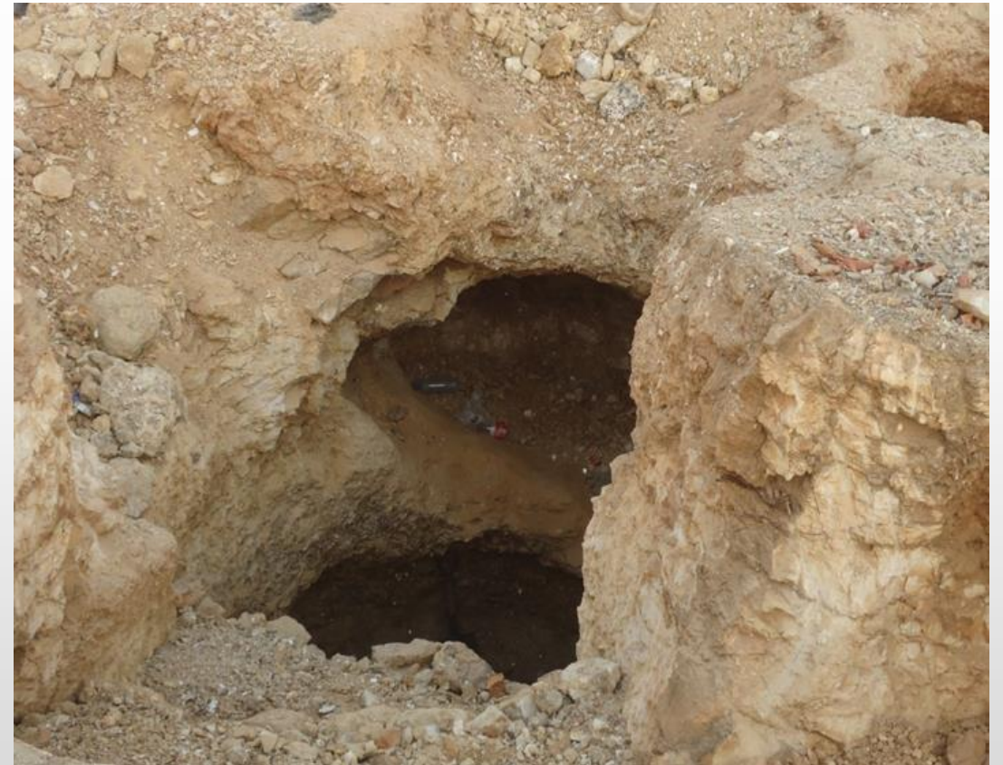
FIGURE: DANGEROUS PITTING BY ARTISANAL MINERS. THE HANGING WALL MAY COLLAPSE ON THEM
