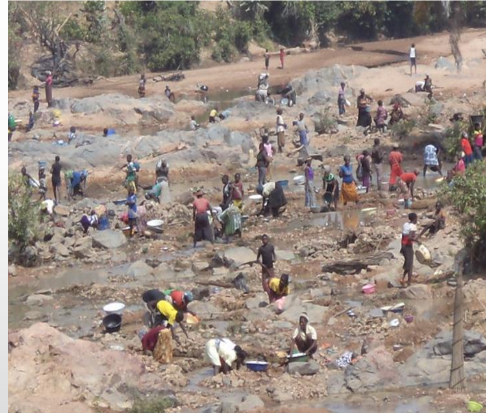
FIGURE: ACTIVE ALLUVIAL TIN MINING IN ARIKPA, NASARAWA-EGGON, CENTRAL NIGERIA. THE LOCAL MINERS SEEN DIGGING AND PANNING FOR THE TIN ORE
