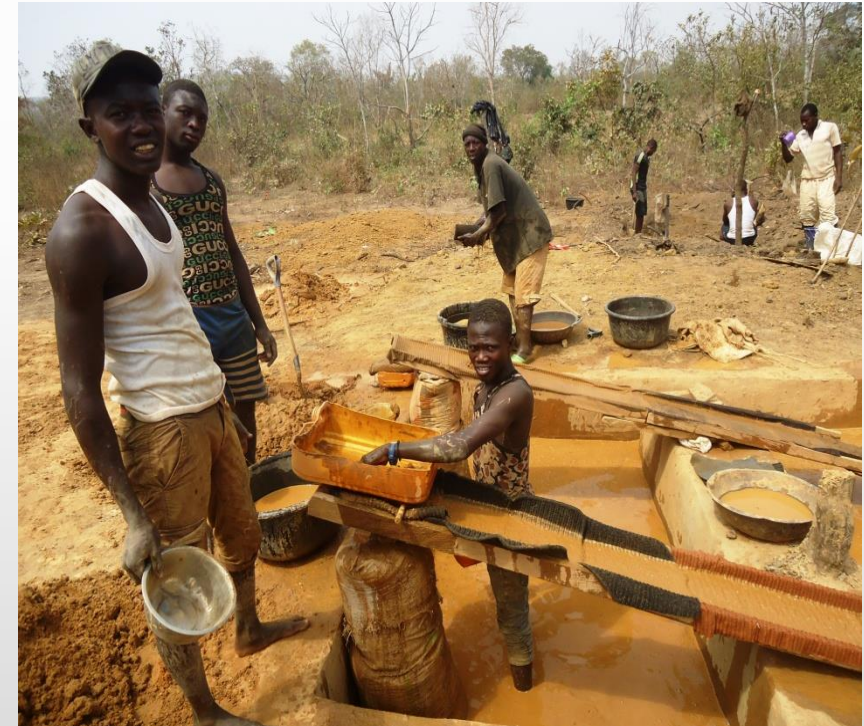
FIGURE: PANINIG AND SLUICING FOR GOLD RECOVERY BY LOCAL MINERS
