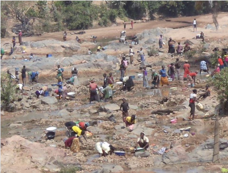
FIGURE : ACTIVE ALLUVIAL TIN MINING IN ARIKPA, NASARAWA-EGGON, CENTRAL NIGERIA. THE ARTISANAL MINERS SEEN DIGGING AND PANNING FOR THE TIN ORE
