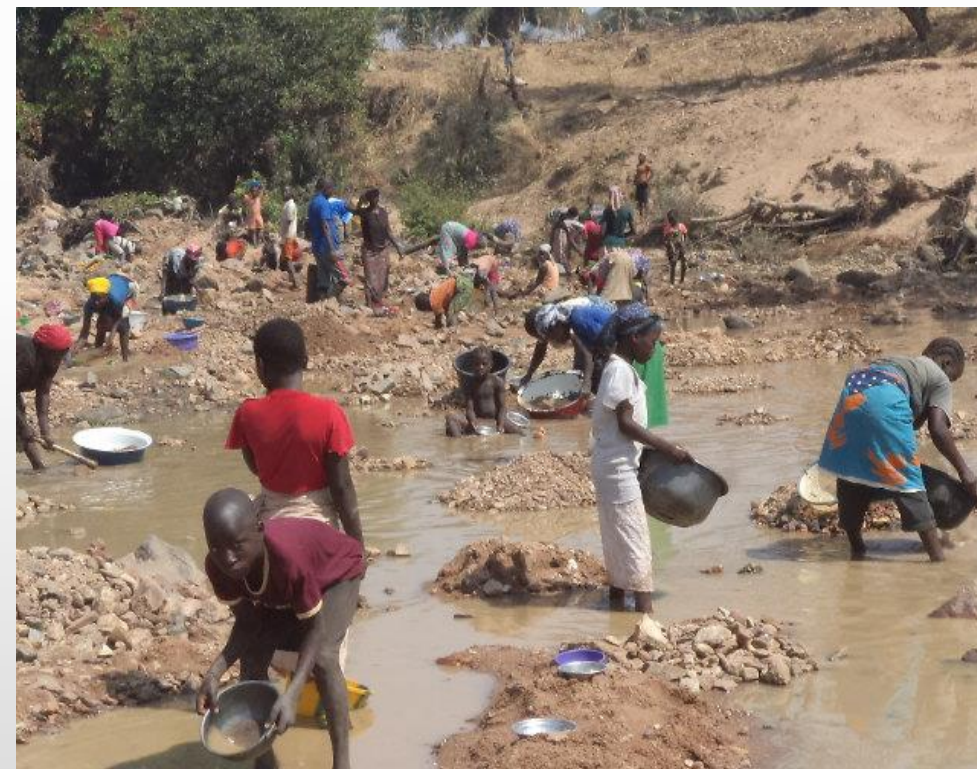
Figure : ACTIVE ALLUVIAL TIN MINING IN ARIKPA, NASARAWA- EGGON,CENTRAL NIGERIA.( CHILDREN MINERS SEEN DIGGING AND PANNING FOR THE TIN ORE )
