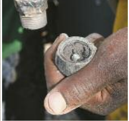
Figure 29 B. The amalgam is placed in the cup of the retort on some ash to get the cup airtight.
