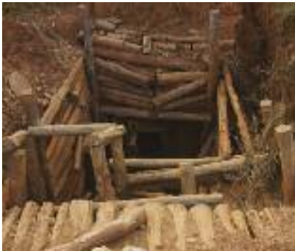
Figure 16. Proposed Underground Mining for ASM Using Vertical Shaft Opening.
