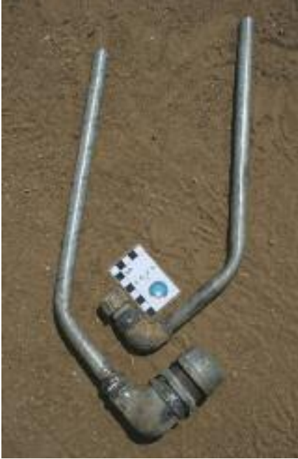
Figure 29 A. Two retorts made of a few pieces of plumbing tubes. The scale is 10 cm.
