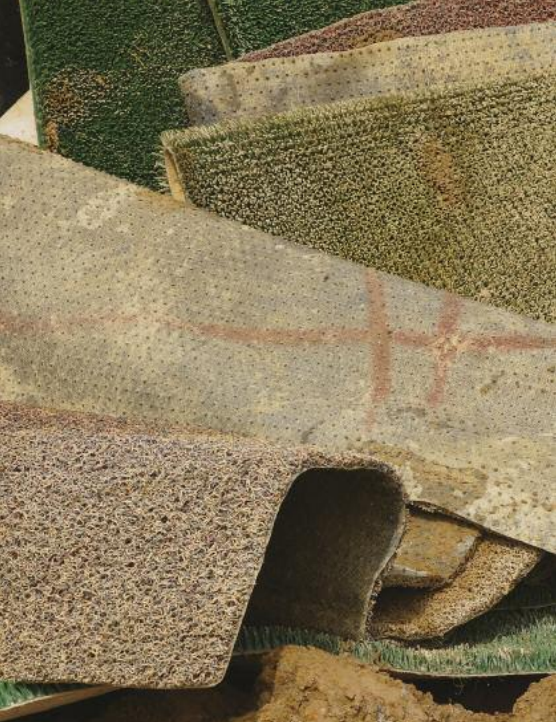
Selection of mats for sluicing, mining site north of Osino in Central Ghana.
