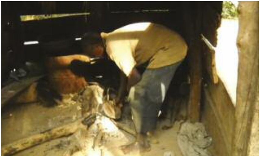
Figure 38. ASM Operator Heating Gold-Mercury Mixture (Amalgam) to Recover Gold.
