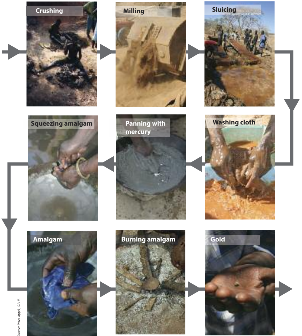
Figure 27. Flowchart. Gold extraction using mercury. Amalgamation Process.
