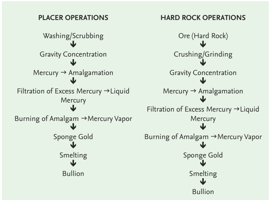
Figure 19. Processing Routes for Placer and Hard Rock Mining Operations.
