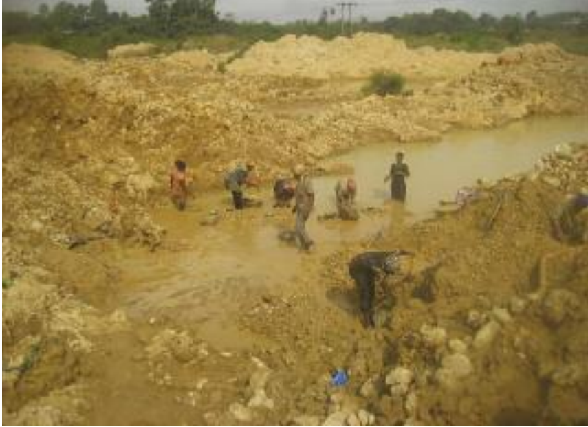
Figure 6. Mining Of An Alluvial Gold Deposit.
