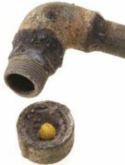
Figure 29 D. Most of the mercury has evaporated and the gold is left behind.
