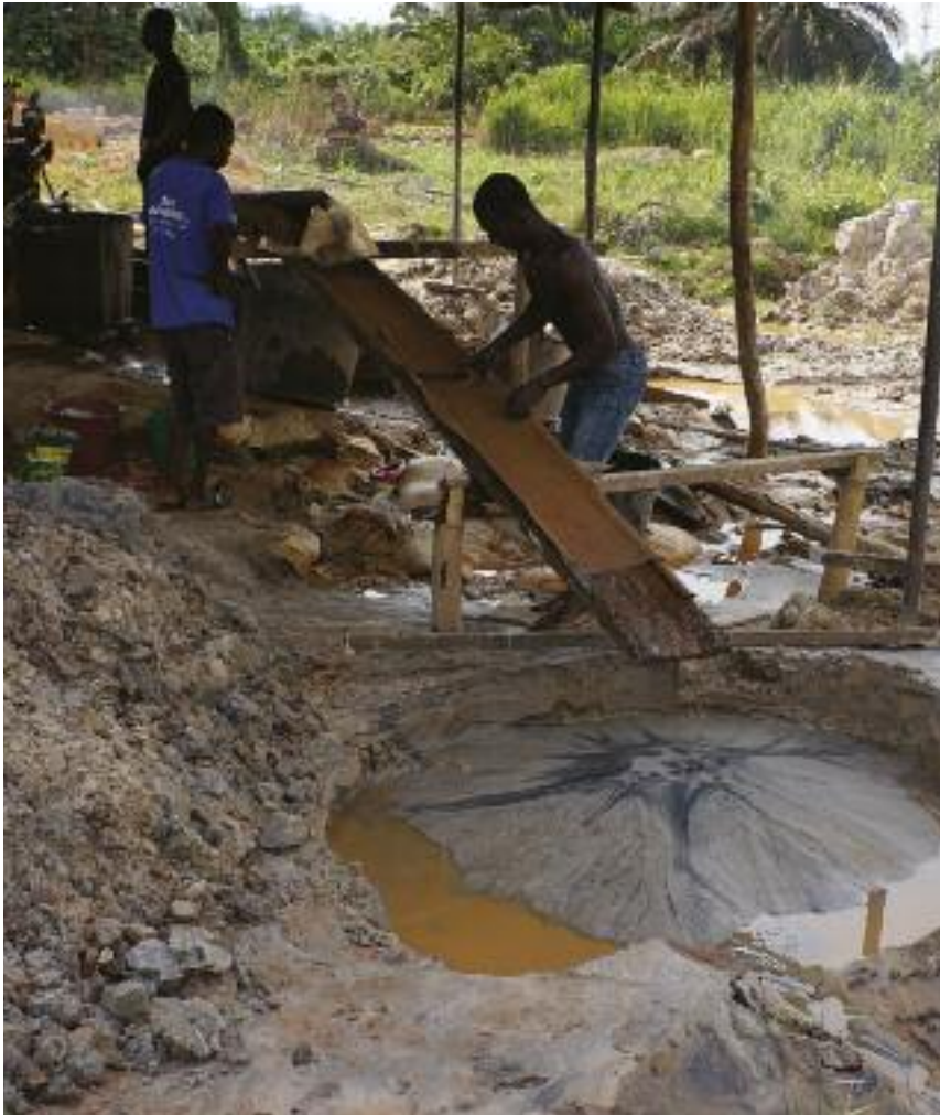
Fig. 24. Sluicing at Artisanal Mining Site North of Tarkwa, Western Ghana.
