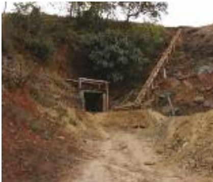
Figure 15. Proposed Underground Mining for ASM Using Adit Method.
