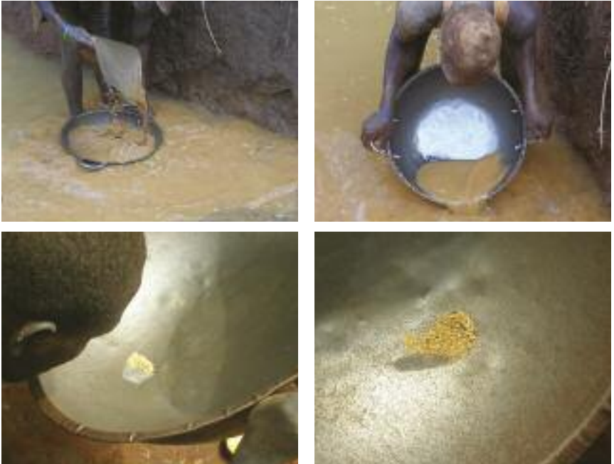
Fig. 25. Goldpanning starting by washing the cloth from the sluicing followed by panning.
